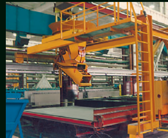
Semi portal frame distributor
