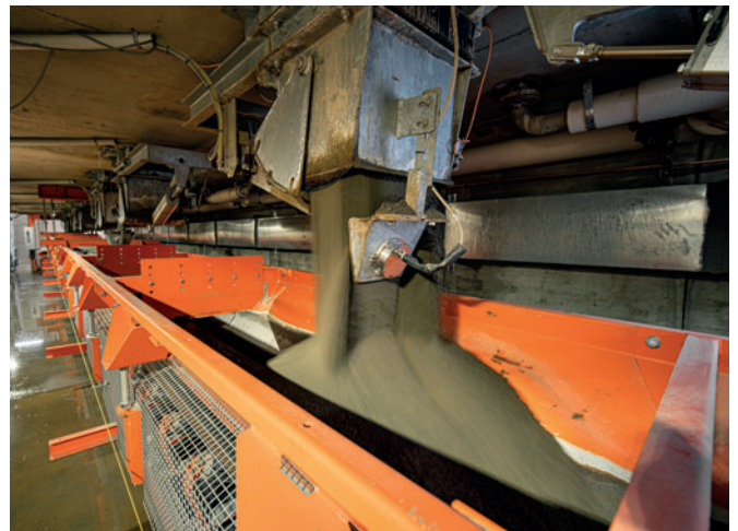
Hydrtester radar moisture probes, mounted below the aggregate batching gates, measure real-time aggregate total moisture. Hydrtester moisture probes are used in the aggregate bins for accurate batch yield correction due to moisture content in the raw materials.
