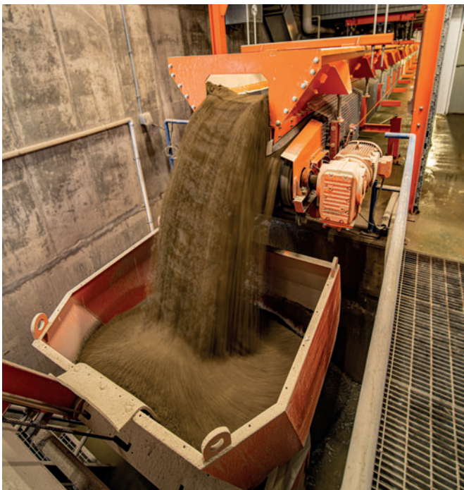
The aggregate weigh belt pre-weighs the next batch into the skip. Pre-weighing and holding the next batch in combination with the high intensity HPGM 2250 mixer maintains fast cycle time so that Camp Precast meets their productivity goals.
